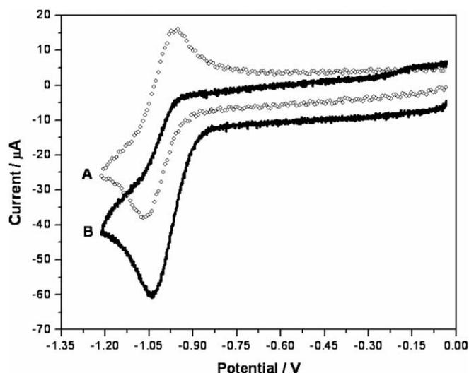
**Fig. 4.** Cyclic voltammograms recorded at a scan rate of  $100 \text{ mV s}^{-1}$  with a freshly polished glassy carbon electrode (area =  $0.071 \text{ cm}^2$ ) in oxygen-free DMF containing  $0.10 \text{ M TBABF}_4$ : (A)  $2.0 \text{ mM}$  nickel(II) diethylsalen; (B)  $2.0 \text{ mM}$  nickel(II) diethylsalen and  $5.0 \text{ mM}$  triclosan. Scans go from 0 to  $-1.20$  to  $0 \text{ V}$ .
