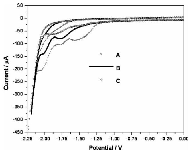
**Fig. 1.** Cyclic voltammograms recorded at a scan rate of  $100 \text{ mV s}^{-1}$  with a freshly polished glassy carbon electrode (area =  $0.071 \text{ cm}^2$ ) in oxygen-free DMF containing 0.10 M TBABF<sub>4</sub>: (A) 5.0 mM triclosan; (B) 5.0 mM 5-chloro-2-(4-chlorophenoxy)phenol; (C) 5.0 mM 5-chloro-2-phenoxyphenol. All scans go from 0 to  $-2.25$  to 0 V.
