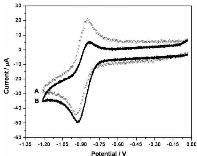
**Fig. 3.** Cyclic voltammograms recorded at a scan rate of  $100 \text{ mV s}^{-1}$  with a freshly polished glassy carbon electrode (area =  $0.071 \text{ cm}^2$ ) in oxygen-free DMF containing  $0.10 \text{ M TBABF}_4$ : (A)  $2.0 \text{ mM}$  nickel(II) salen; (B)  $2.0 \text{ mM}$  nickel(II) salen and  $5.0 \text{ mM}$  triclosan. Scans go from 0 to  $-1.20$  to  $0 \text{ V}$ .
